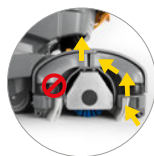
Alternate twin squeegee system (patented)
