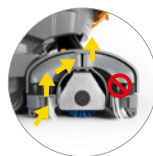
Alternate twin squeegee system (patented)
