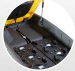
Recovery tank lifting system: easy access to the vac motor and to the battery compartment.
