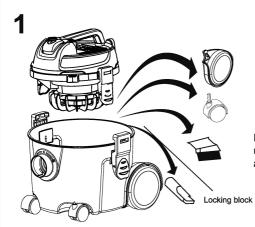
Release the lock block to open the up housing, take out wheels and accessories.
