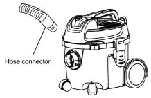
Insert the hose connector into the swivel of the Vacuum Cleaner.
